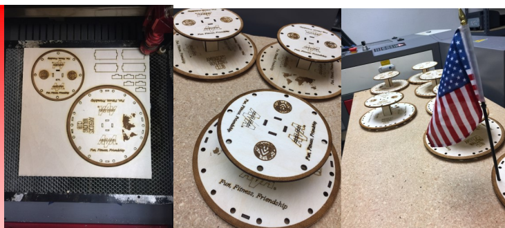
Flag stands being made by Hector with the laser engraver for the Texas Trail Roundup.
